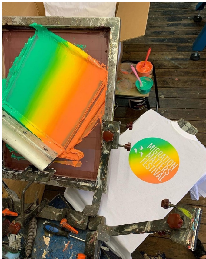
Keep the screen flooded with ink between prints when screen printing water-based inks. @hunkprint
